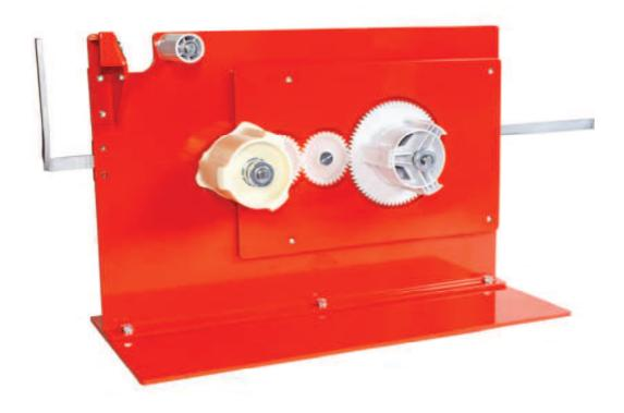
It is a bench dispenser for easy use of double-sided tapes or single-sided adhesive tapes with a protective liner (ex. aluminium tapes) up to 250mm of external diameter. It is designed for industrial use, where large quantities of tapes are used and efficiency is the main request. The dispenser removes the liner and rewinds it on a spool, giving the peeled off tape ready to use. It permits saving a lot of time.
