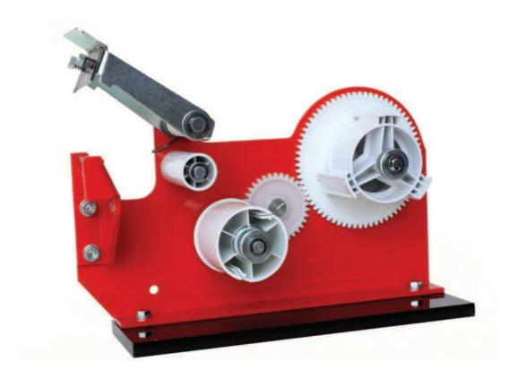
It is a bench dispenser for easy use of double sided tapes or single-sided adhesive tapes with protective liner. It is designed for the use of tapes that the toothed blade cannot cut. The dispenser removes the liner and rewinds it on a spool, making the peeled off tape ready to use. It is an useful tool that permits saving a lot of time when using double-sided tapes.
