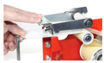
This particular execution is characterized by an additional sliding arm. This permits cutting pieces of tape at a pre-set length . The maximum length is 500 mm.
