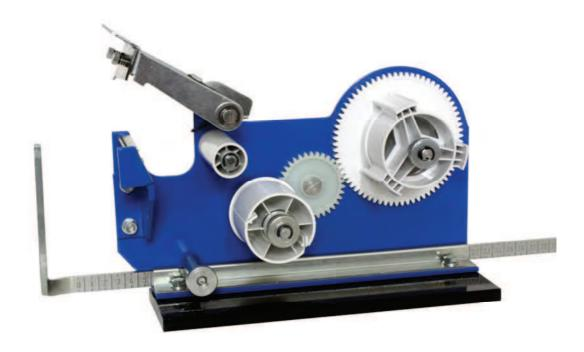
It is a bench dispenser for easy use of double sided tapes or mono-adhesive tapes with protective liner. Designed to use tapes that the toothed blade cannot cut. The dispenser removes the liner and rewinds it on a spool, making the peeled off tape ready to use. It is an useful tool that permits saving a lot of time when using double-sided tapes.
