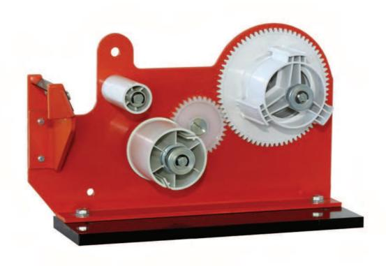
It is a bench dispenser for easy use of double-sided tapes or single-sided adhesive tapes with a protective liner. It is used to make paper or cardboard self-adhesive, stick parts on sample books and assemble parts. The dispenser removes the liner and rewinds it on a spool, making the peeled off tape ready for use. It is an useful tool that permits saving a lot of time when using double-sided tapes.
